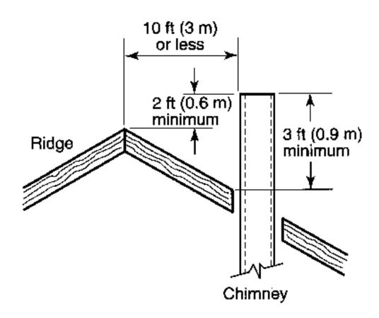
**B**) If the flue terminates beyond 10 feet from the ridge of the roof, the flue must simply clear the upper penetration of the roof by 3 feet. Notice, however, that the flue still terminates 2 feet above the roof at the 10 foot perimeter:
