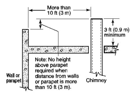
D) In this flat roof example, the same rules apply. In the diagram below, the flue on the right terminates within 10 feet of the parapet, so it must terminate 2 feet above the parapet height, as in Diagram B above. Notice the left flue on the neighboring building: it also terminates 2 feet above that same parapet, since it is also within 10 feet of that parapet:
